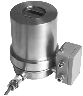
RHE 11 Explosion Proof Version Protection Class: EEX de {ia} IIC Explosion Proof Class I, Division 1, Group C & D, pending. Power Supply: 110/220V AC (50/60 Hz): 24V DC
